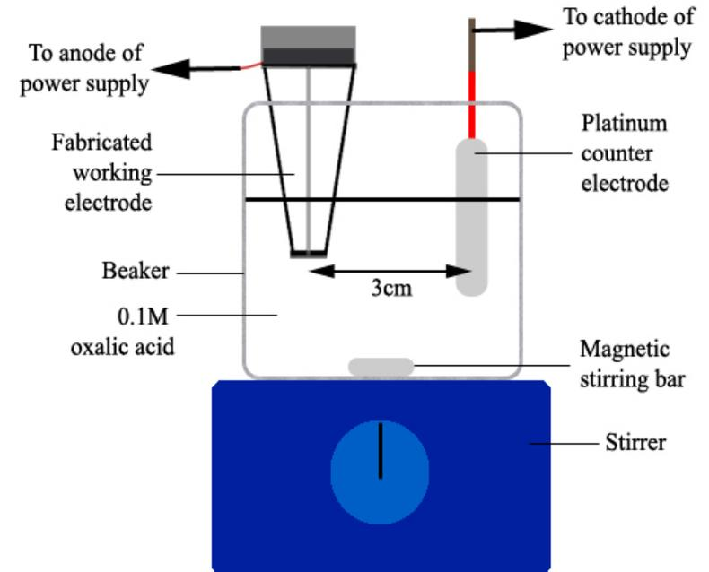
**Left:** Schematic of fabrication of electrode using *surface contact pipette* anodization method
