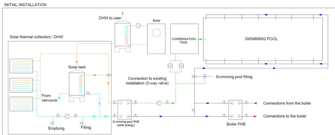
Figure 2. Schematic of the initial installation at the Aljorra swimming pool.
