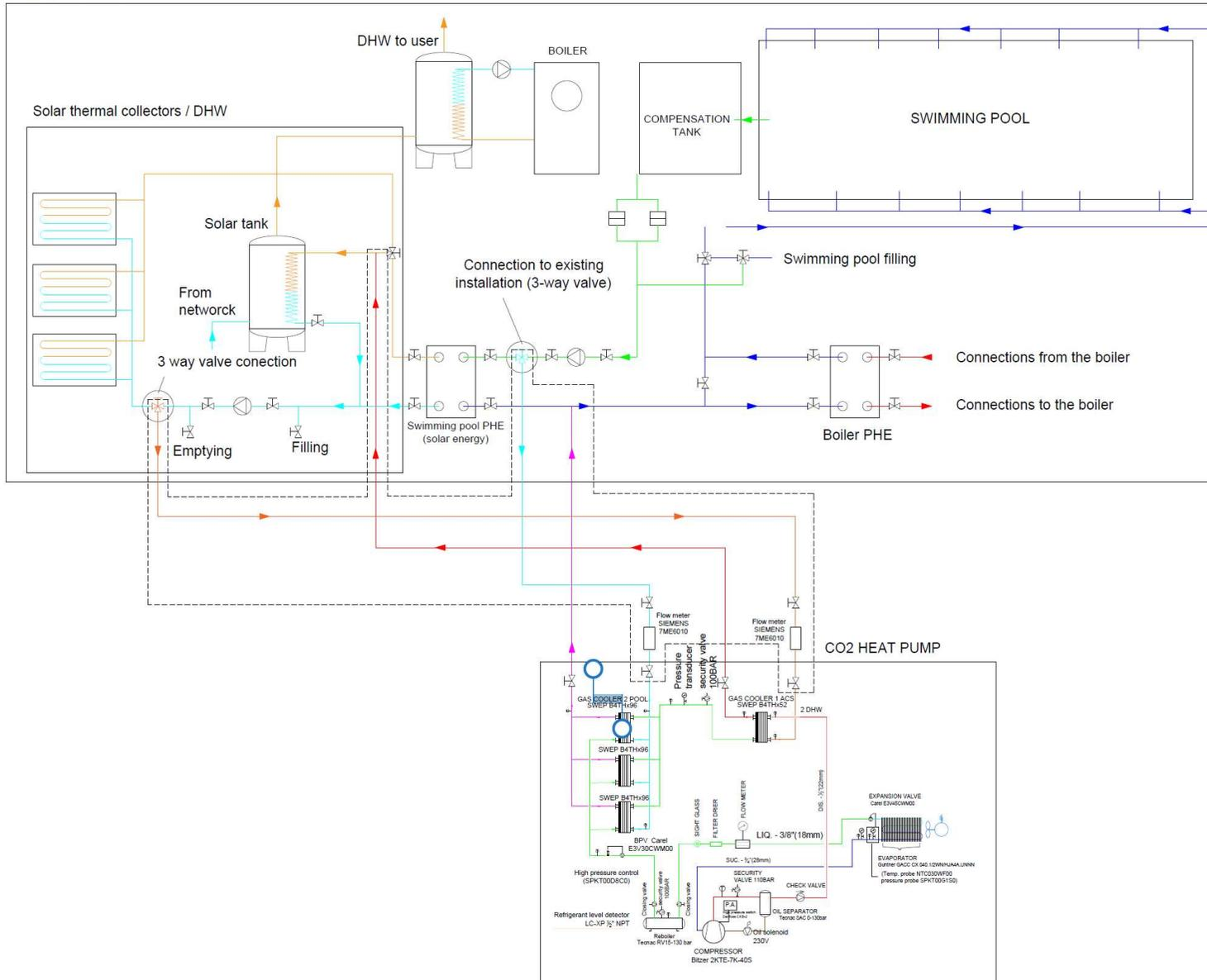
Figure 3. Installation including the heat pump.
