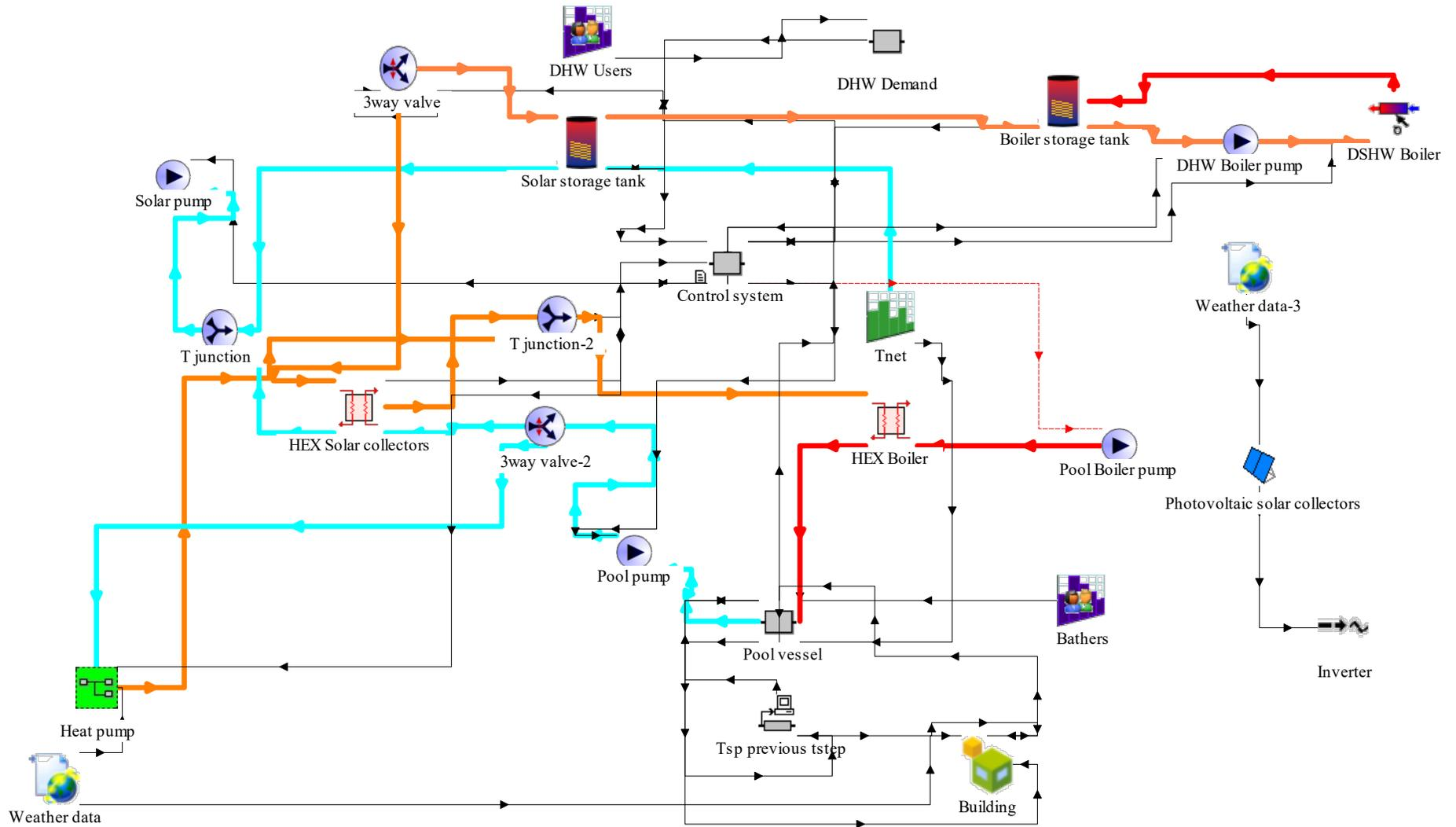
Figure 6. TRNSYS model of the swimming pool facility including the heat pump.
