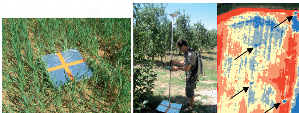
Fig. 10. Aluminium targets – Position measurement – Targets seen as cold points on thermal image.
