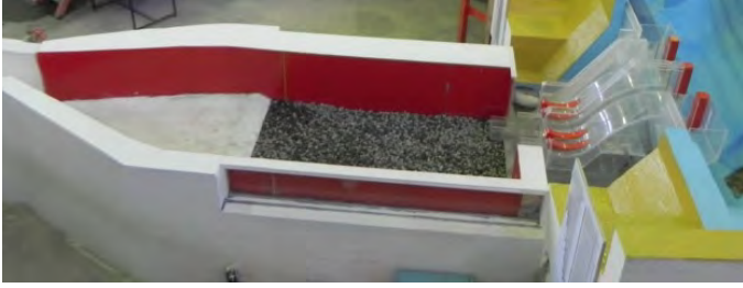
Figure 2. Physical model of the Toachi sky jump.
