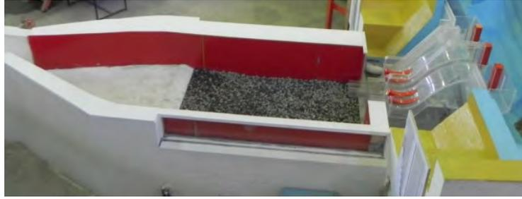
Figure 27. 1:50 scale physical model of the Toachi ski jump (EPN 2013).
