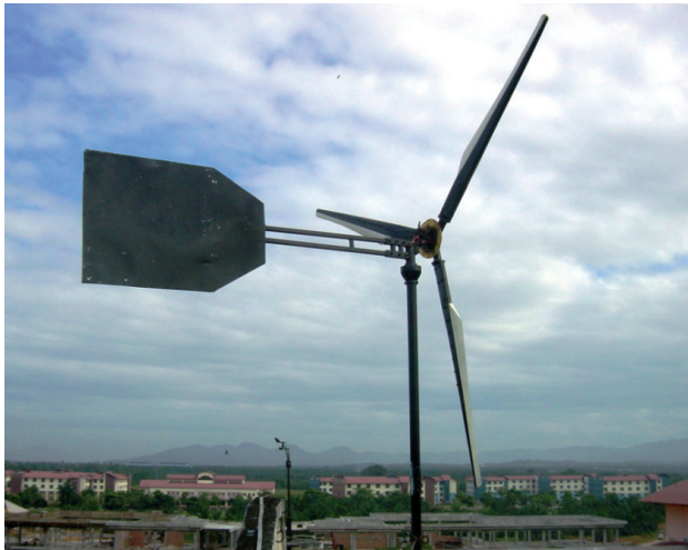
Figure 10. Wind turbine with optimized generator during turbine evaluation. Notice the anemometer in the background to the left.
