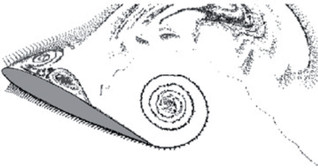
Figure 9. Aerodynamic stall mechanism – Vortex shedding at the trailing edge
