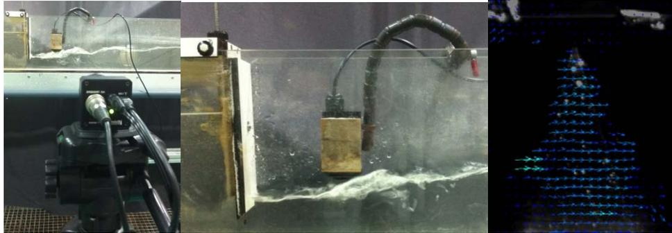
Figure 2. PIV instrumentation position and detail of post processing velocity vectors
