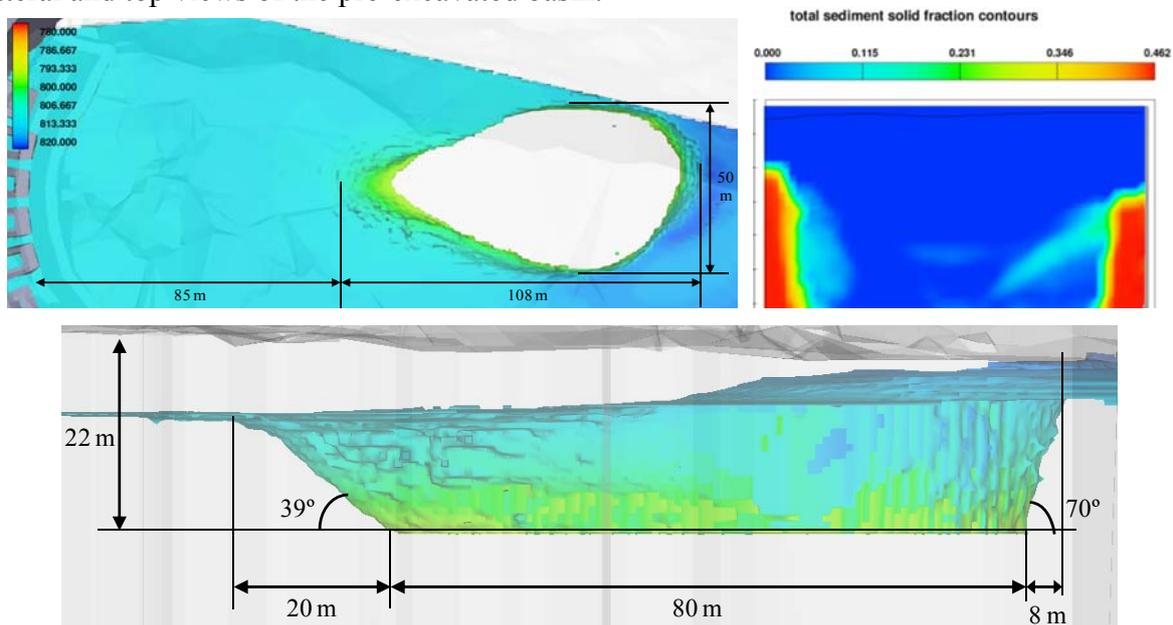
**Figure 11:** Top, front and lateral views of the scour due to the half-height outlet
