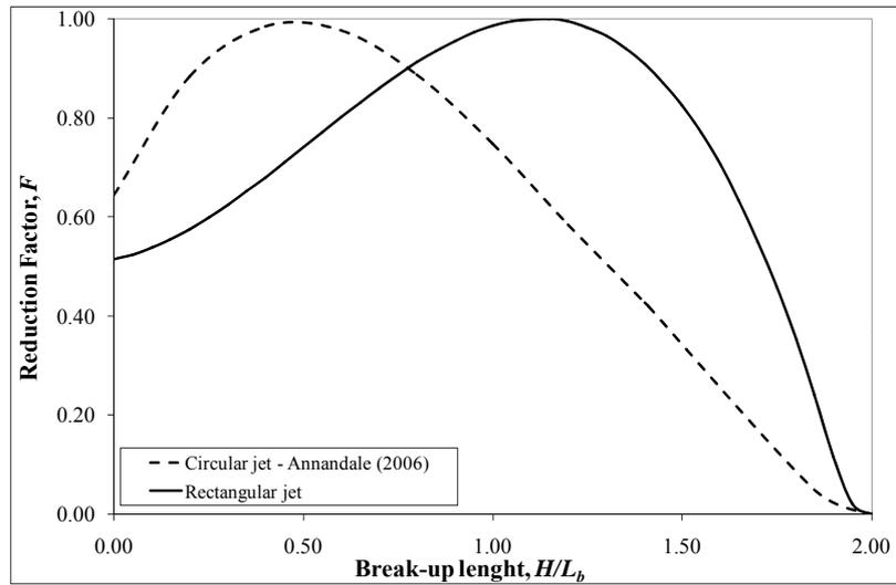
Figure 6: Reduction factor  $F$  of fluctuating dynamic pressure coefficient
