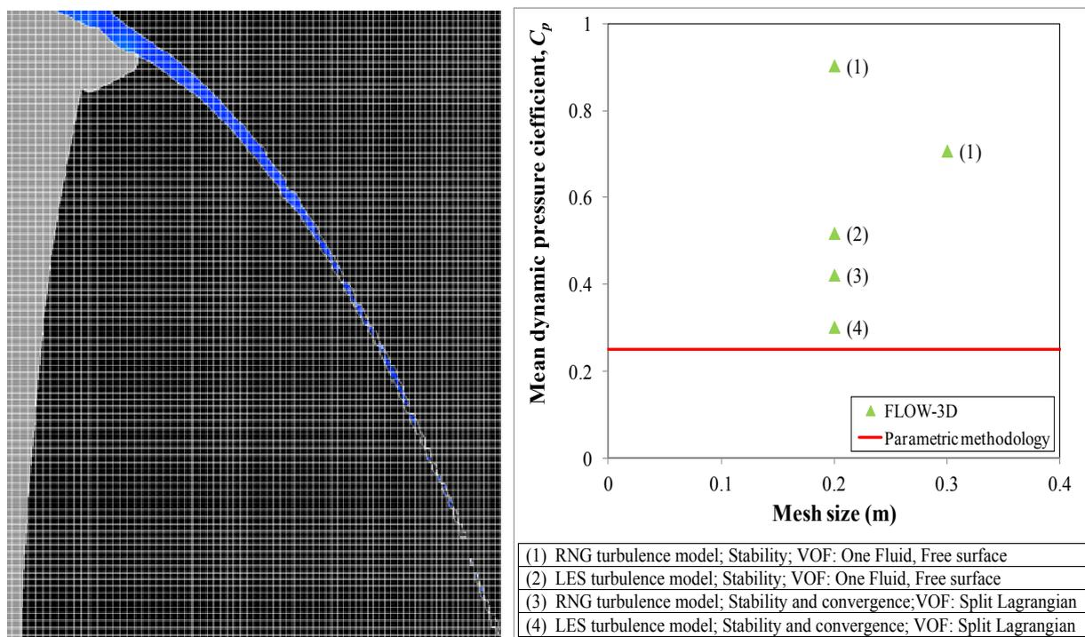
**Figure 9:** Mesh and sensibility analysis of FLOW-3D
