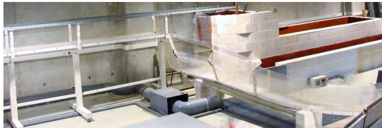
Figure 1. Physical model of the bottom rack intake built in the Hydraulic Laboratory of the Universidad Politécnica de Cartagena.
