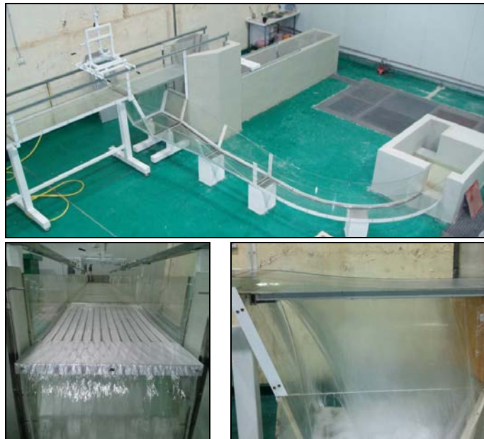
Figure 1 Device of intake system of the Hydraulic Laboratory of Universidad Politécnica de Cartagena, Spain
