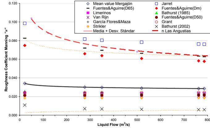
Figure 8. Manning resistance coefficient  $n$  versus flow rate. Mergajón and Las Angustias gullies.
