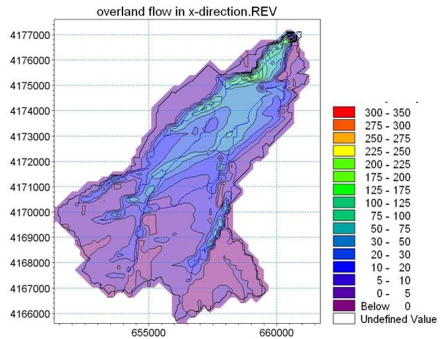
Figure 5. Maximum overland flow in x direction for T500 years.
