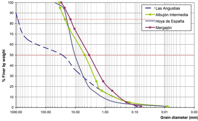
Figure 7. Grain-size distribution curves of the gullies.
