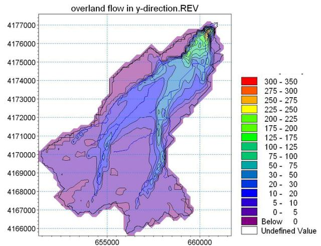
Figure 6. Maximum overland flow in y direction for T500 years.
