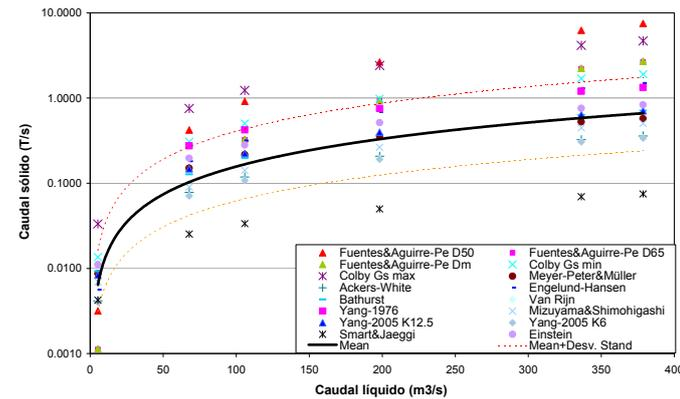
Figure 9. Solid flow versus liquid flow in Albujión Intermedia gully.
