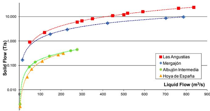
Figure 10. Total bed transport in function of liquid flow.
