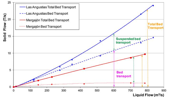
Figure 11. Total bed transport in function of liquid flow.
