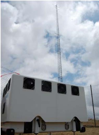
Fig. 1. Equipment at test site: WindCube (front) and Met Mast (back)
