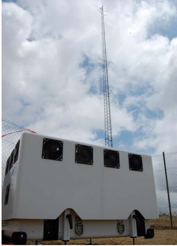
Figure 1. Equipment at test site: Lidar (front) and Met Mast (back)
