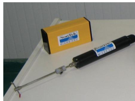
Figura 3.6. Sonda y receptor ADV
