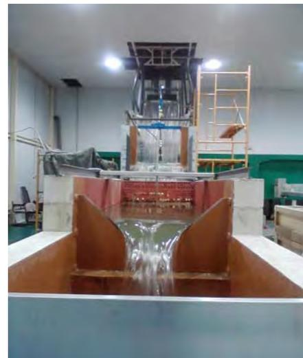
**Figura III.7: Vertedero triangular de pared delgada.**
