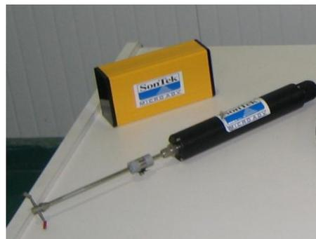
**Figura 3.6. Sonda y receptor ADV**
