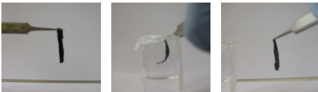
Fig. 1. Optical images of bending-recovery behaviour (a) original shape (b) bending in acetone vapor (c) recovery in air
