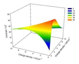
Contrast plot of a seven layer configuration electrochromic device, as a function of the redox charge of its electroactive constituent materials. Maximum contrast conditions are clearly identified. Results shown correspond to a poly-3,4ethylenedioxy-thiophene (PEDOT)/ poly-3,6-bis(2-(3,4-ethylenedioxy)thienyl)-N-methylcarbazole (PBEDOT-NMCz) dual polymer system, at a fixed wavelength of 555 nm.
