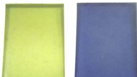
Figure 1 Bleached and colored states of a dual polymer electrochromic device, composed of PEDOT and PBEDOT-NMCz
