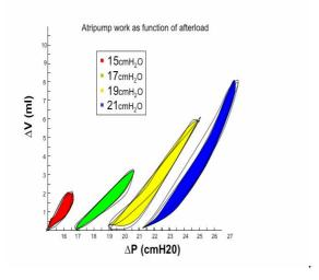
The contraction rate was 1Hz with power supply of 12V, 400mA for 200ms. Pre-load ranged from 15 to 21cmH2O. Graphic resumes pressure volume relationship. Maximal silicone membrane temperature was 55  $\,\mathrm{C}^{\circ}$  and maximal temperature of the liquid environment was 35  $\,\mathrm{C}^{\circ}$ .
