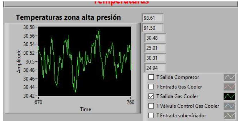
Fig. 37. Refrigerant temperature out of the gas cooler with 0.15 K oscillation.
