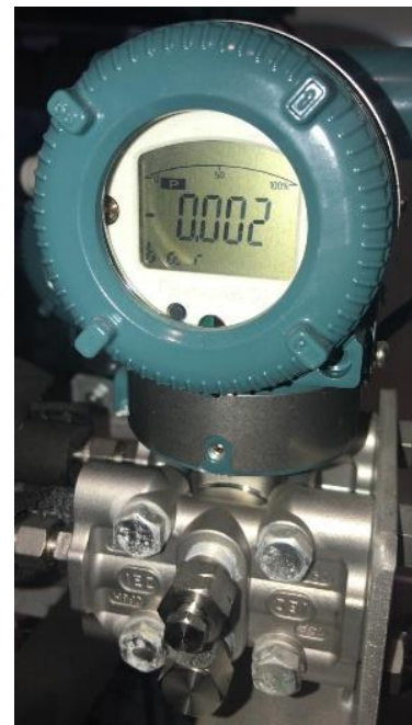
Yokogawa, EJX 110A. Differential pressure
