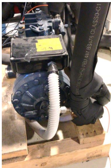
(b) Suction line and power input
