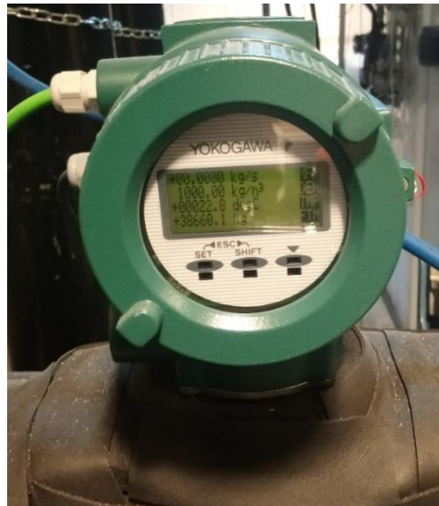
Fig. 28. Coriolis effect refrigerant mass flow meter.
